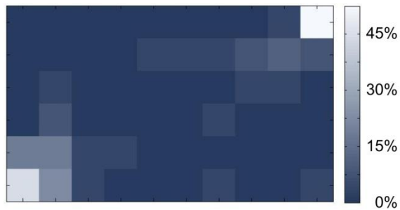
Figure 7: Percentage of cells cracked in the 45° direction at each position in the cell matrix.
