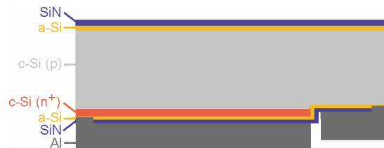
Figure 1 Schematic of the cross section of half of a unit cell. The drawing is not to scale.
