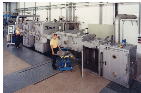
Figure 6: In-line high-rate coating equipment "MAXI" at Fraunhofer FEP Dresden
