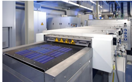
Fig. 1: ATON 500 inline high-rate evaporation system installed at the ISFH.
